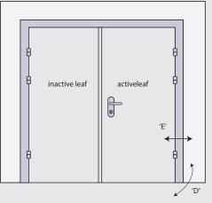
may require packing shims to maintain the position (not supplied) Both sides of the frame may require adjustment. Open the door leaf, make the adjustments and close to check the door is hanging true.
